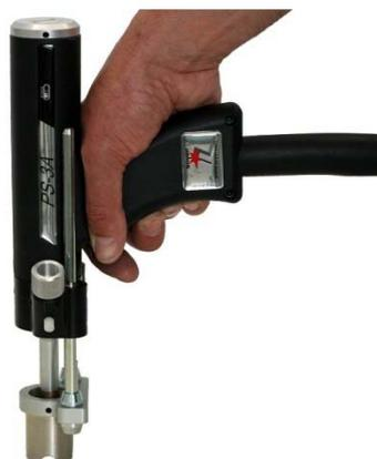
Position welding gun vertically on the workpiece (at a 90-degree angle to the workpiece). Check once again the selected parameters. Release welding process by pressing the push button.
