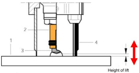
**Adjusting and checking the height of lift**
