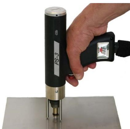
Position welding gun vertically on the workpiece (at a 90-degree angle to the workpiece). Check once again the selected parameters. Release welding process by pressing the push button.
