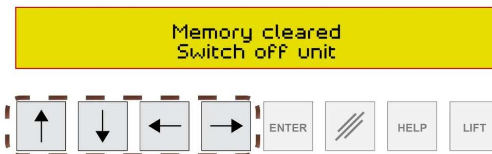
Switch off the stud welder with main switch and switch on again.
