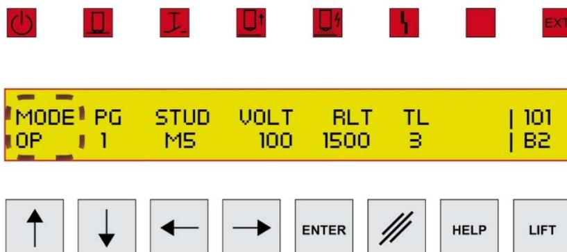
Example of a display shown after stud welder has been switched on:
