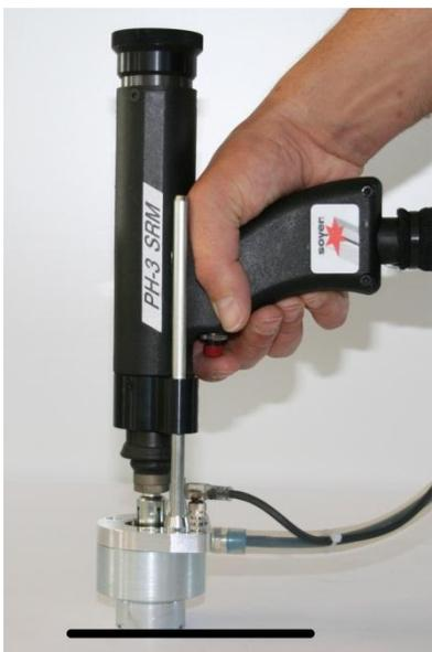
Position welding gun vertically on the workpiece (at a 90-degree angle to the workpiece).
