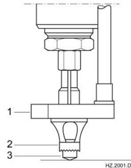
Fig. Stud welding with ceramic ferrule
