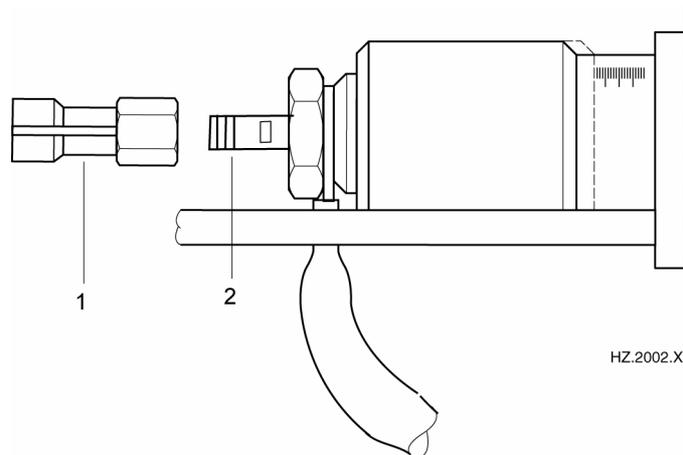
The stud holder (1) must be tightly screwed on the retaining screw (2). When the screwed connection is not tight enough, these parts could be damaged by scorching during the welding process.
