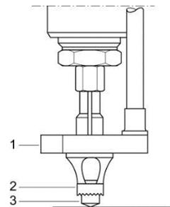
*Illustration: Stud welding with ceramic ferrule*
