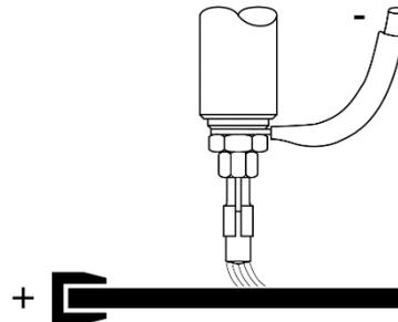
Additional masses disturb arc symmetry.
