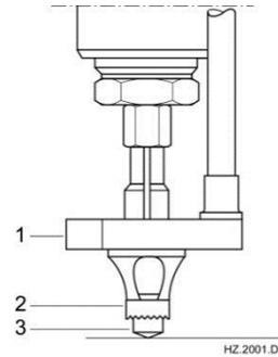
Fig. Stud welding with ceramic ferrule
