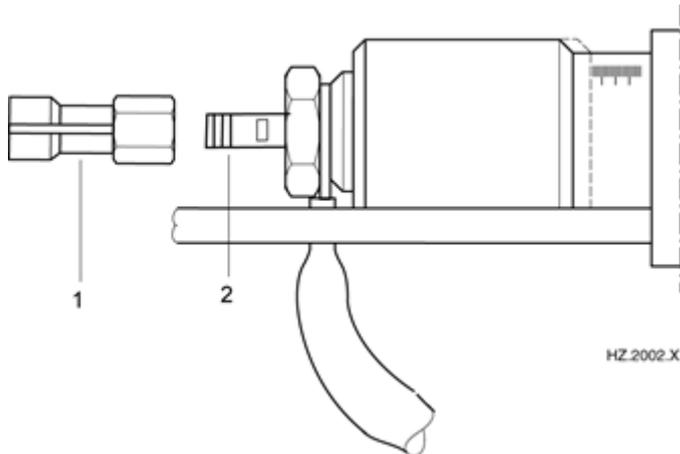
The stud chuck (1) must be tightly screwed on the retaining screw (2). When the screwed connection is not tight enough, these parts could be damaged by scorching during the welding process.
