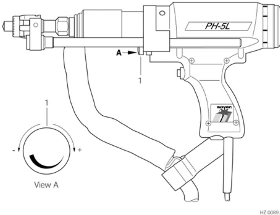
The immersion speed or its damping depends on the stud diameter.
