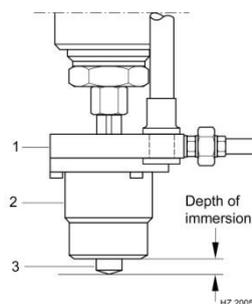
Fig. Stud welding with shielding gas
