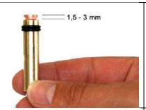
Ensure depth of immersion / stud protrusion is set between 1.5 mm and 3 mm.
