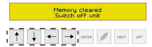
Switch off the stud welder with main switch and switch on again. The stud welder is now operative.
