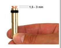
Ensure depth of immersion / stud protrusion is set between 1.5 mm and 3 mm.
