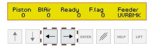
The parameters "Piston", "Ready", "F.lag." and "BlAir" may be selected in 100 ms steps. The parameters may be horizontally selected by using the function keys "Arrow left" and "Arrow right".
