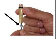
The weld stud must make contact with the stop screw. Adjust stop screw in the stud chuck by turning it until the distance between the top edge of the stud flange and the front edge of the stud chuck equals 1.5 mm.
