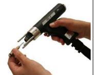
The stud welder must be <u>switched off</u> when installing the stud chuck.
