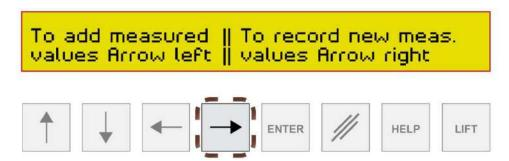
Call the option "Record new measured values" by pressing the "Arrow right" key.
